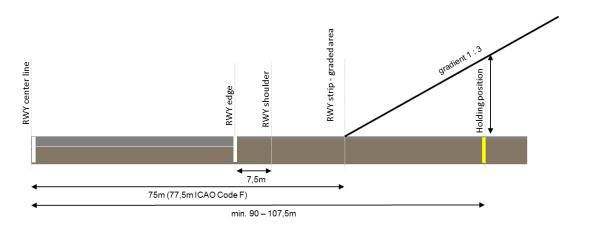
The obstacle free zone (OFZ) – gradient 1:3 – shall be free of temporary and fixed objects during CAT II / III operation on the runway. The graded area of the runway strip must be constructed, as followed:
