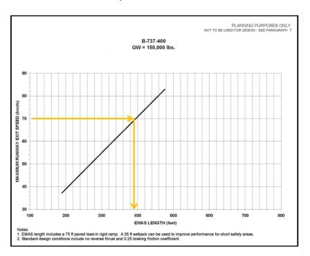
$\underline{Origin:}$  (AC 150/5220-22B) – Example B737-400 with runway exit speed of 70 knots = EMAS length 395 ft
